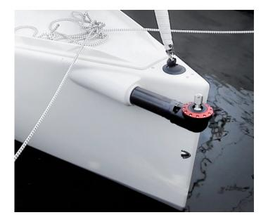
The new battery-powered, remote control, E-Furler from LOOP® Products – designed to make life simpler and more enjoyable.
